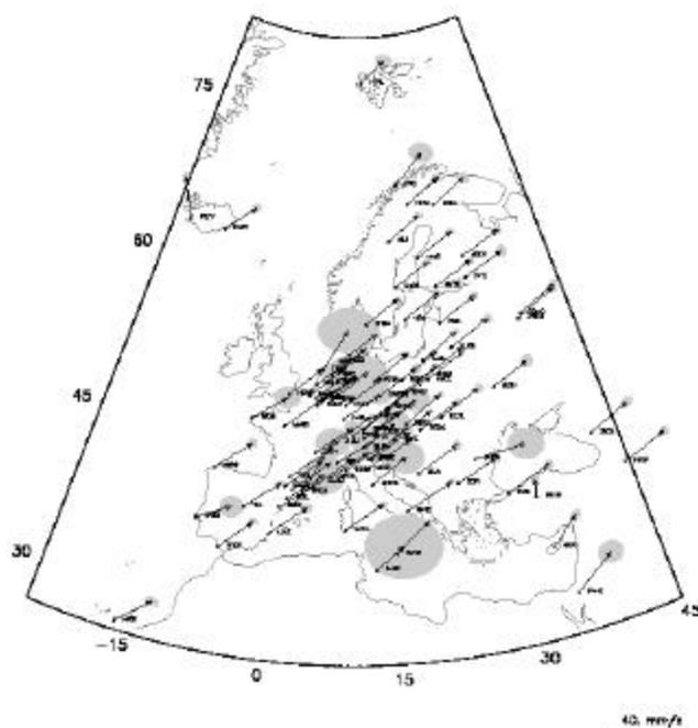
**Figure 3** Velocities of the unconstrained solution for the EUREF contribution to ITRF2000. Formal error ellipses are scaled by a factor of 15 for the plot.
