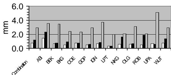
**Figure 2.** Average rms values of the weekly EPN combinations solutions for the 1999 and individual LAC rms (north, east, up). Average rms for the combinations is 0.7, 1.2 and 3mm for the north, east and up components.
