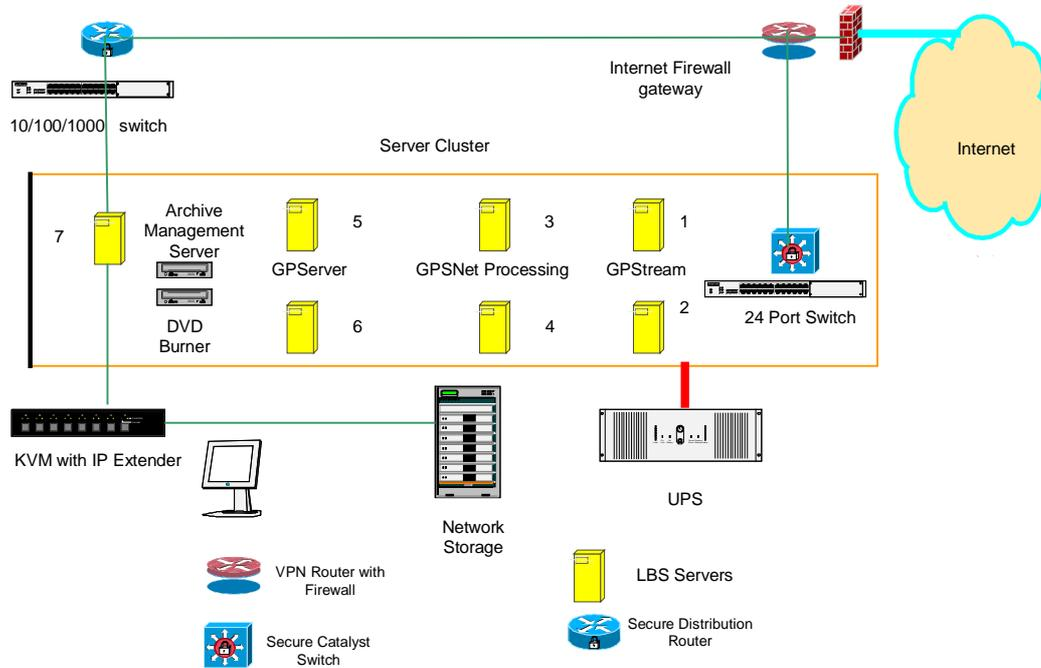
**Figure 4.** Data Centre Schematic (Adapted from Trimble 2004)
