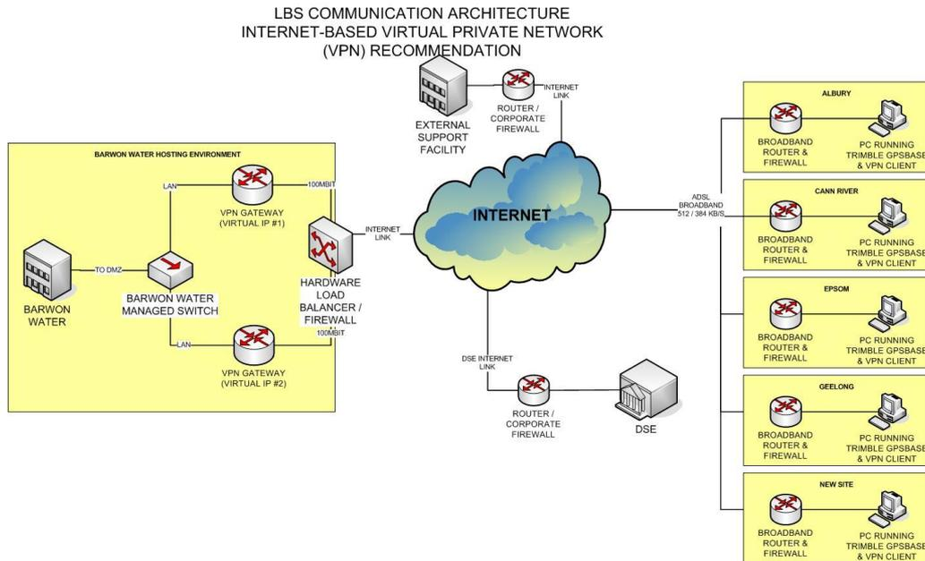
**Figure 2.** Internet based VPN model (Geomatic Technologies 2004)
